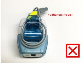
DO NOT wrap the cable around the optional pole mount in any manner.
