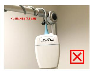
DO NOT coil the sensor cable around a ventilator circuit support arm, monitor stand, or any object less than 3 inches [7.6 cm] in diameter.
