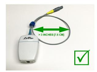
Always coil the cable in the direction of the natural cable coil, greater than 3 inches [7.6 cm] in diameter. The use of cable ties is acceptable, and will aid in maintaining the diameter of the cable during storage. Position the cable tie to avoid sharp kinks at the connector and sensor strain reliefs.
