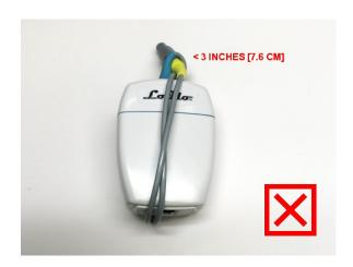
DO NOT wrap the cable around the sensor in any manner.
