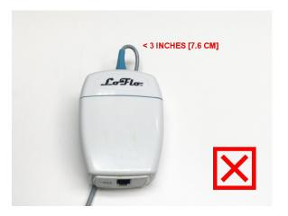
DO NOT kink the sensor cable, or bend the sensor cable less than 3 inches [7.6 cm] in diameter.
